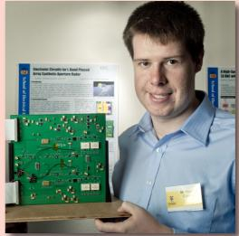
Thomas Cooney's final year research project was to design a signal processing board for the satellite's radar antenna. He worked with the radar designers at Astrium in the UK to identify all requirements, then designed the board. When built, the board was successful on the first try. Thomas has finished his degree and is working for an Australian biotechnology company.
