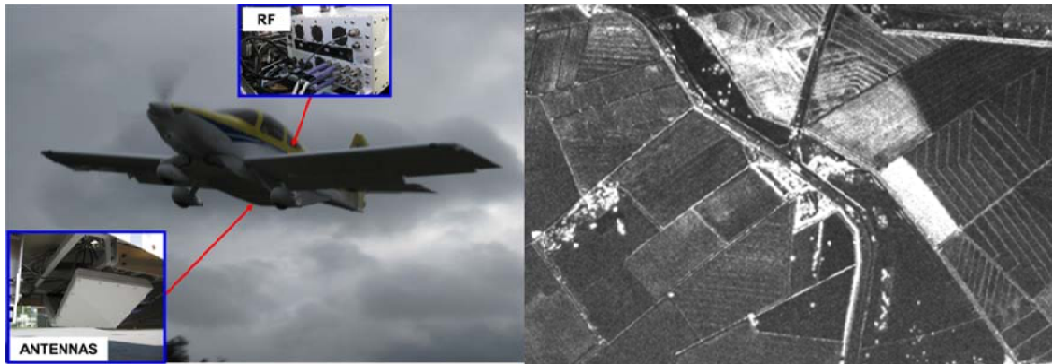
Figure 10.3 The Polarimetric L-band Imaging Synthetic Aperture Radar (PLIS) on an Australian aircraft (left) and a sample image from the Yanco study area (right) that is shown in Figure 10.2.
